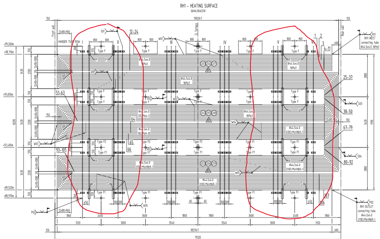
Picture 4: Hanger tubes partial replacement areas
